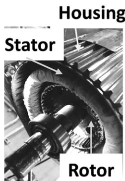
Fig. 1 Photograph of fabricated 5 kW class HTS-ISM
