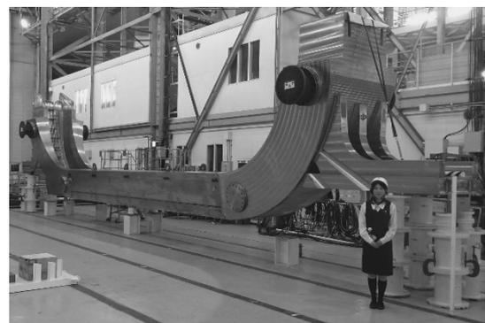
Fig. 3 Overview of AU main structure
