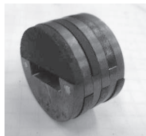
Fig.1 Undulator magnet array using MgB 2 superconducting bulk magnets.
