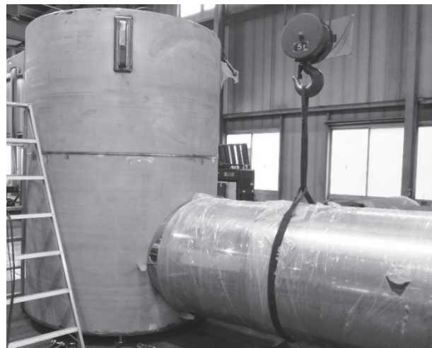
Fig.2 Vacuum Chamber Assembly of CTB for PF Coils
