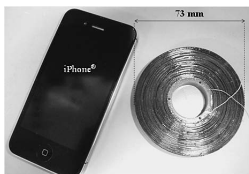
Fig.1 A 73 mm outer diameter pancake coil wound with a PIED YBCO-coated conductor impregnated with epoxy.
