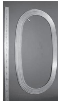
Fig.1 Photograph of impregnated racetrack coil
