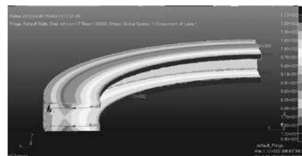
Fig. 3 Circumferential stress of bonded structure
