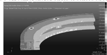
Fig. 4 Circumferential stress of screwed structure
