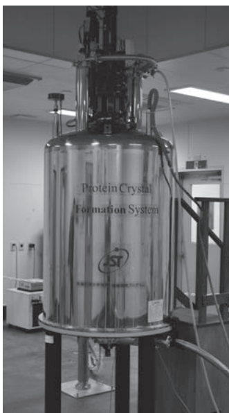
Fig. 1 A photograph of the superconducting magnet for the protein crystal formation system.
